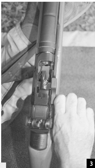
1. Poke a round into the chamber. 2. Unlatch the magazine. 3. Let the bolt halfway home and then release it. 4. Relatch the magazine.
