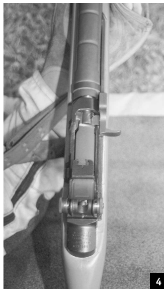
1. Poke a round into the chamber. 2. Unlatch the magazine. 3. Let the bolt halfway home and then release it. 4. Relatch the magazine.
