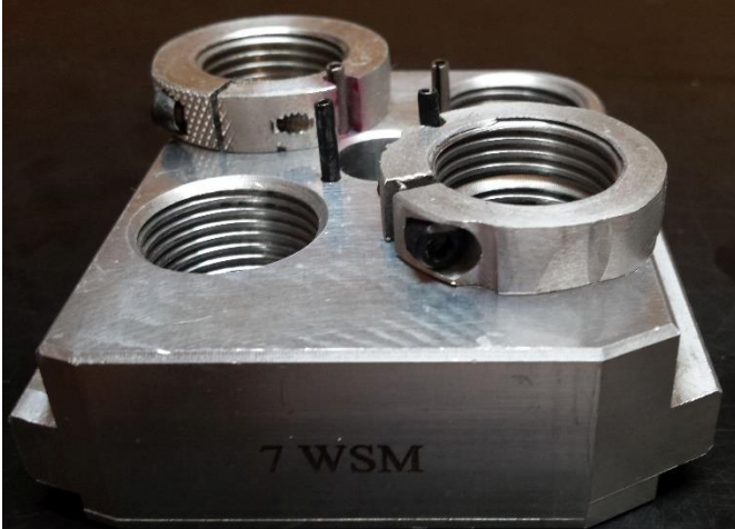
Uniquetek/Whidden Floating Die Toolhead
