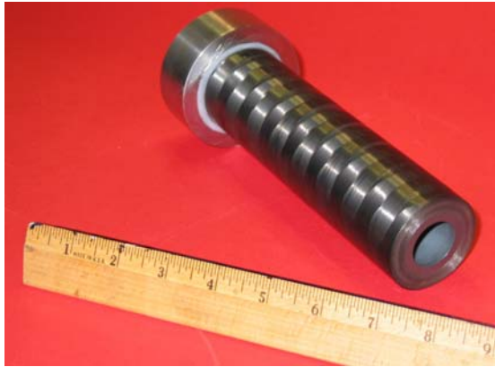
Figure 4 – Overwrapped ceramic tube for ballistic testing.
