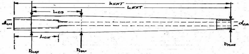
The mass of the barrel  $M_{\text{bar}}$  ahead of the receiver face is then calculated from its total steel volume and the input density  $\rho$  for that type of barrel steel. We use the externally measured barrel length  $L_{\text{ext}}$  for vibration calculations. [The internal rod-measured barrel length  $L_{\text{int}}$  is needed for QuickLOAD] So, before considering any possible muzzle attachments, we start with:
