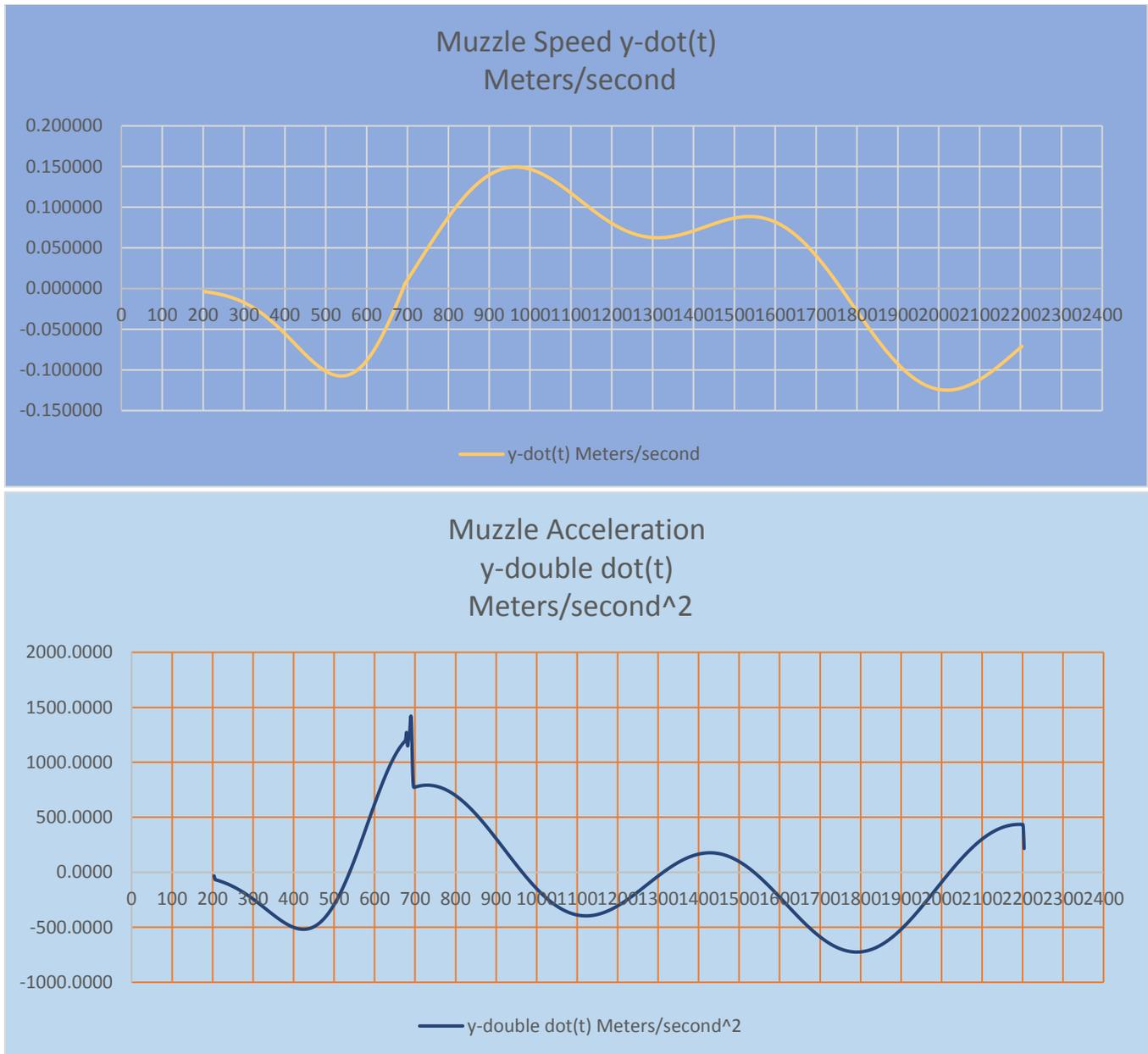
The step-discontinuity in muzzle lateral acceleration is a formulation artifact caused by suddenly switching from recoil-forced distortion of the barrel to damped ringing at the instant of peak muzzle disturbance at  $t = 700$  **microseconds** here. No actual rifle bullet could exit the muzzle of a **25.5-inch** barrel anything like this quickly. Note that the peak upward acceleration of the muzzle is an impressive **125 "G's"** of **9.80665 m/sec<sup>2</sup>** each in this example.
