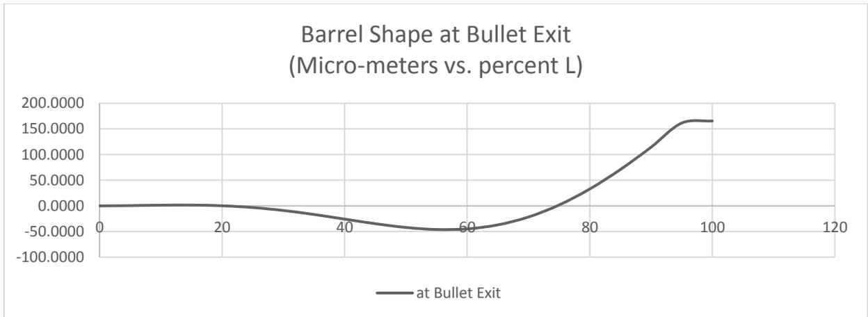
Of course, the vertical scale is greatly exaggerated here relative to the horizontal scale. The horizontal “tail” shown here to the right of the muzzle position at about **96-percent** of **L** is an artifact of Excel’s curve-fitting and of my limited Excel programming skills.
