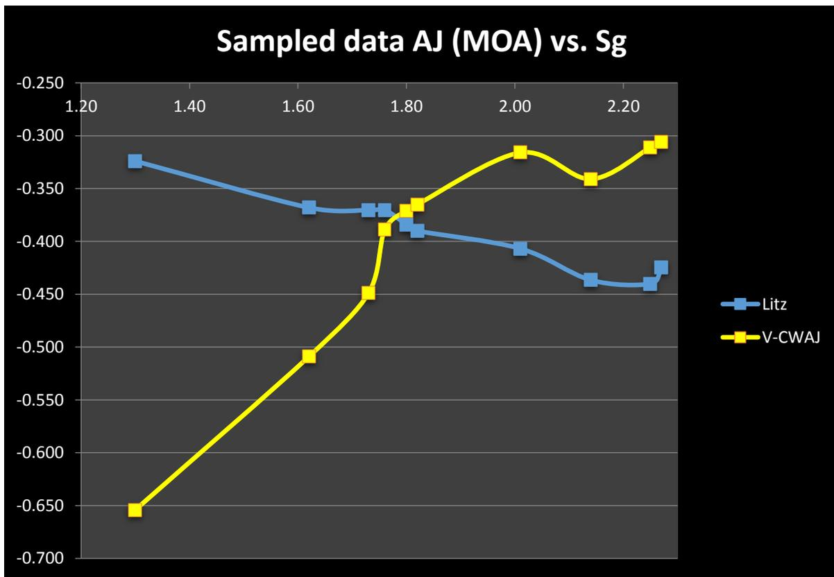
The following chart shows how each method responds to a varying  $S_g$  (also called **stability factor**); it's clear that in the Litz method linear dependency on  $S_g$  is extremely high.
