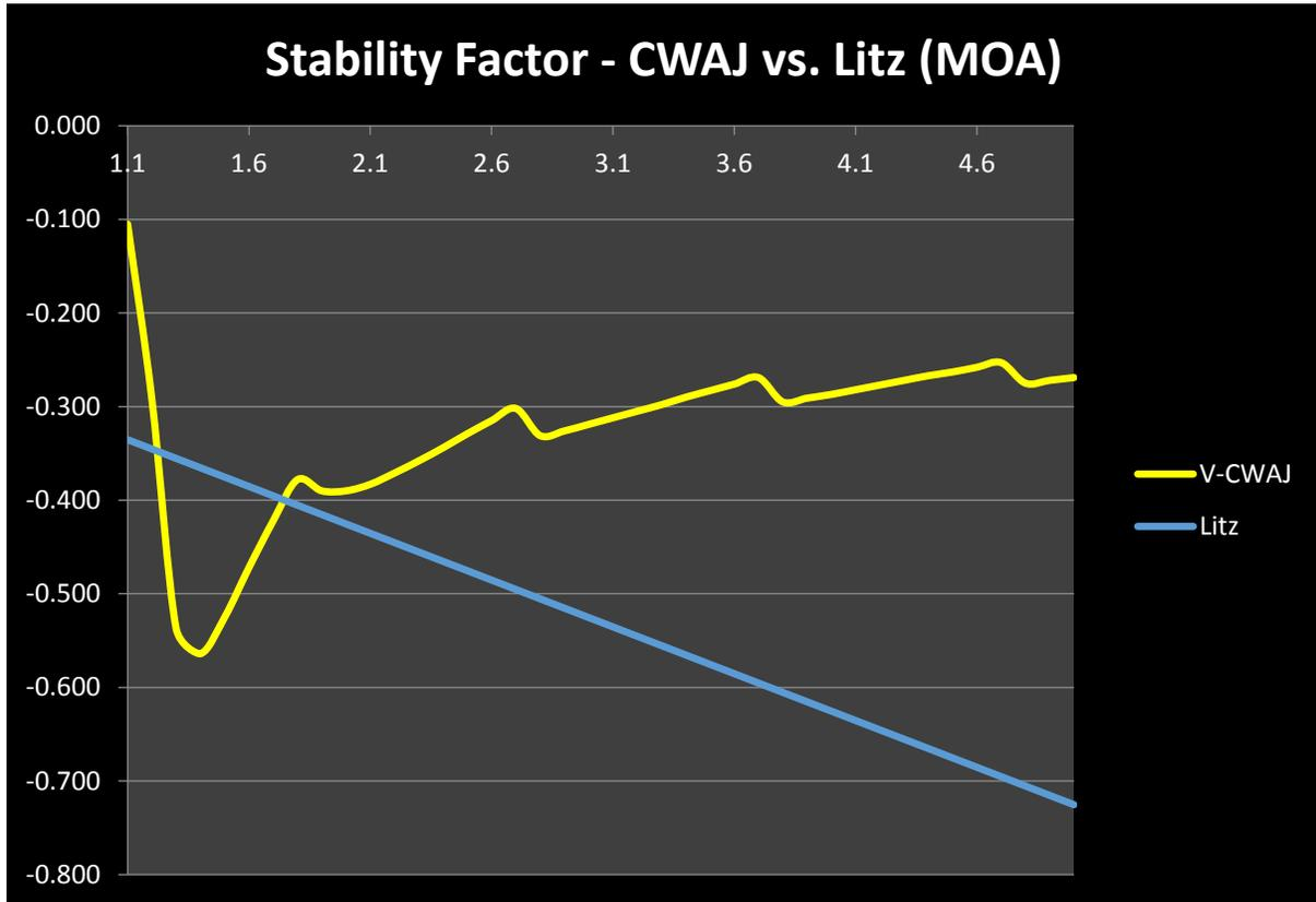
Therefore, if the bullet under study has a resulting  $S_g$  close to 1.75, the “sweet spot” resulting from the original fitted dataset, Litz’s method can provide a fair estimate.
