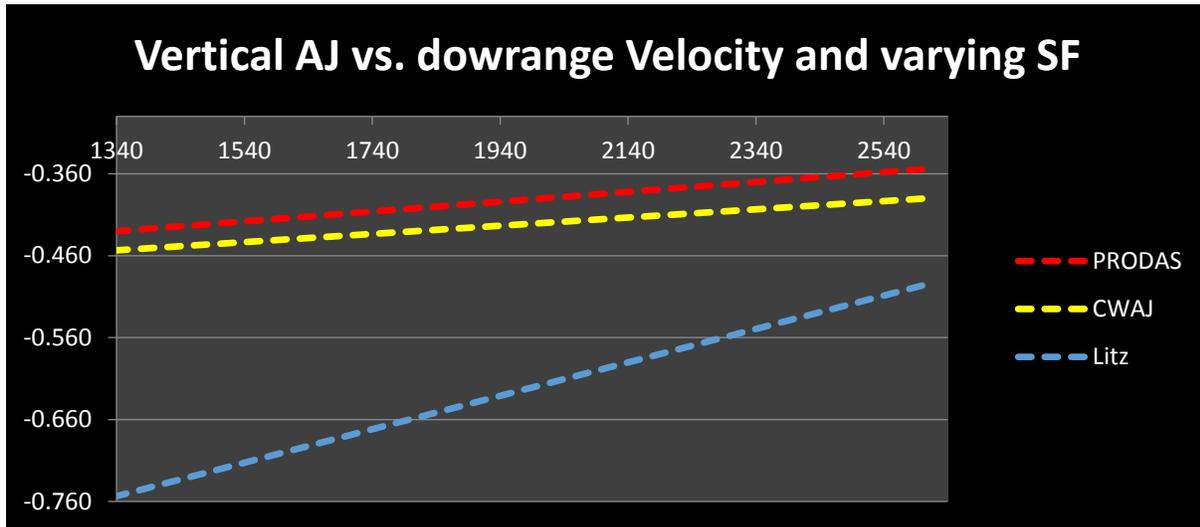
The Standard Deviation is 2.5% for the **CWAJ** model and 12.9% for the Litz's estimator, percentages that given the linearization remains the same for the next dataset.
