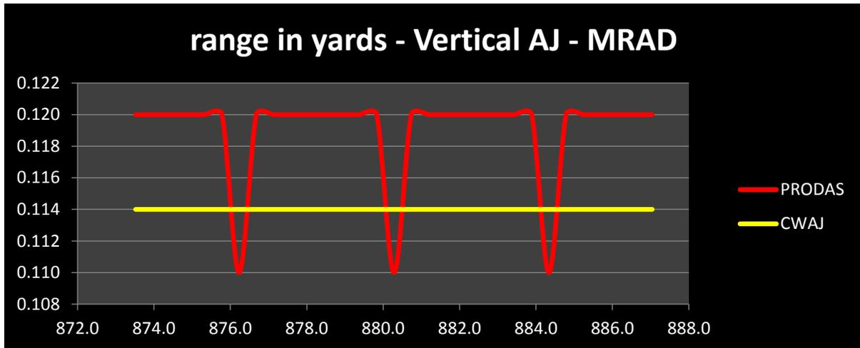
The PRODAS CWAJ-V data are derived by differencing the **DROP** values of the CG from the bore axis, point by point, for two back-to-back PRODAS runs differing only in the constant crosswind value: 10 MPH constant Left-to-Right crosswind versus No Wind, each with the same right-hand rifling twist.
