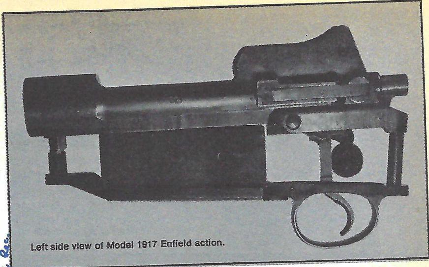
trigger guard, and is secured by a small spring-loaded latch in the guard just to the rear of the magazine box opening. Depressing this latch with a pointed tool, through a hole in the rear of the floorplate, allows the latter to be moved back and released.
