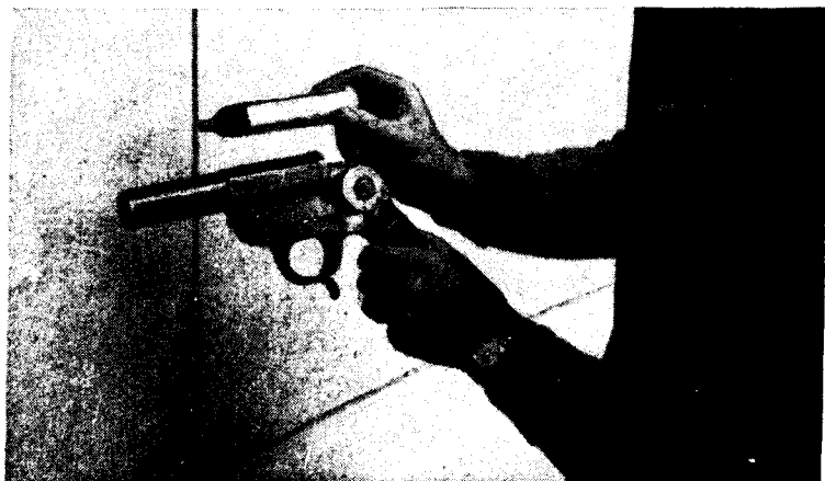
Figure 17.—Pistol grenade being breech-loaded.
