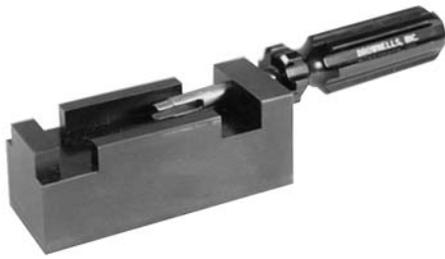
Brownells Ruger Mainspring Pusher is used to compress the mainspring and detent ball on Ruger Mk I and Mk II Auto pistols to remove the housing latch lever, retaining pin and mainspring. This is necessary when rebluing the gun or replacing the mainspring when tuning the action.
