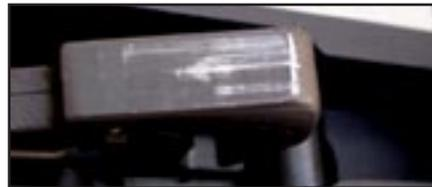
Wear on top of hammer where bolt carrier makes contact.
