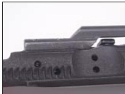
With less than 1,000 rounds fired, carrier key on this bolt is starting to show wear. If it shines, it needs lubrication.
