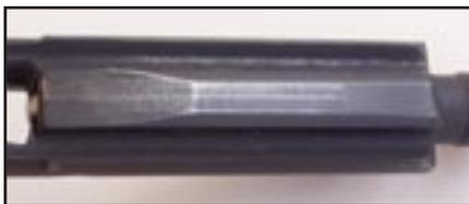
Wear area on bottom of bolt carrier needs lubrication.
