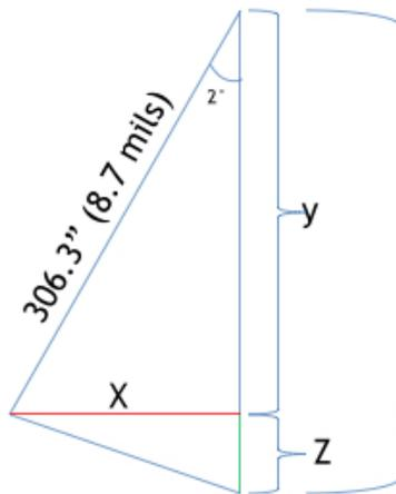
Had the rifle and scope been level this dimension would have been 306.3" (8.7 mils), therefore Z represents the vertical offset error when a  $2^\circ$  rifle/scope cant error is induced by the shooter.
