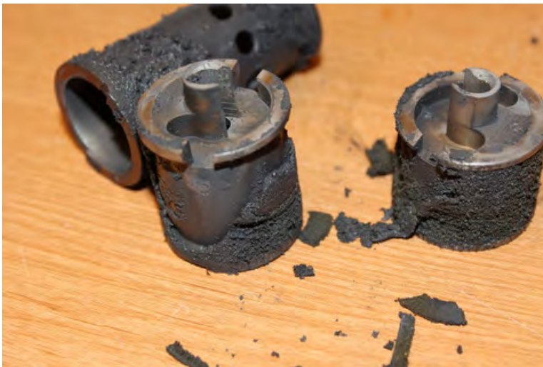
HTG Silencer I-7 core after 1200 rounds of 17 HMR
