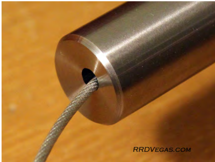
The cable can damage a crown if pulled through at an angle.
