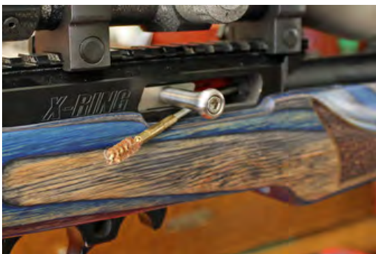
Feed the cable through the ejection port.
