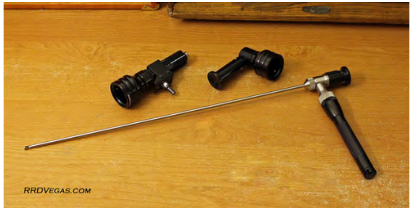
Borescope, Sony camera, and angled eye piece.
