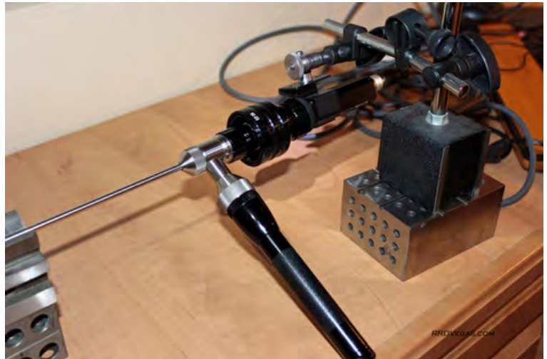
Sony camera hooked up to the borescope.
