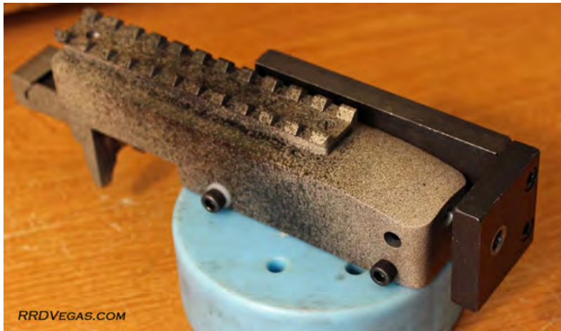
Receiver Drilling Jig
