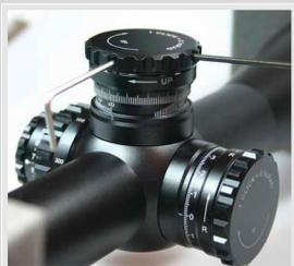
Reinstall the knob and keep in mind to position the two screws at 3 and 6 o'clock. Press the knob firmly against the air resist-
