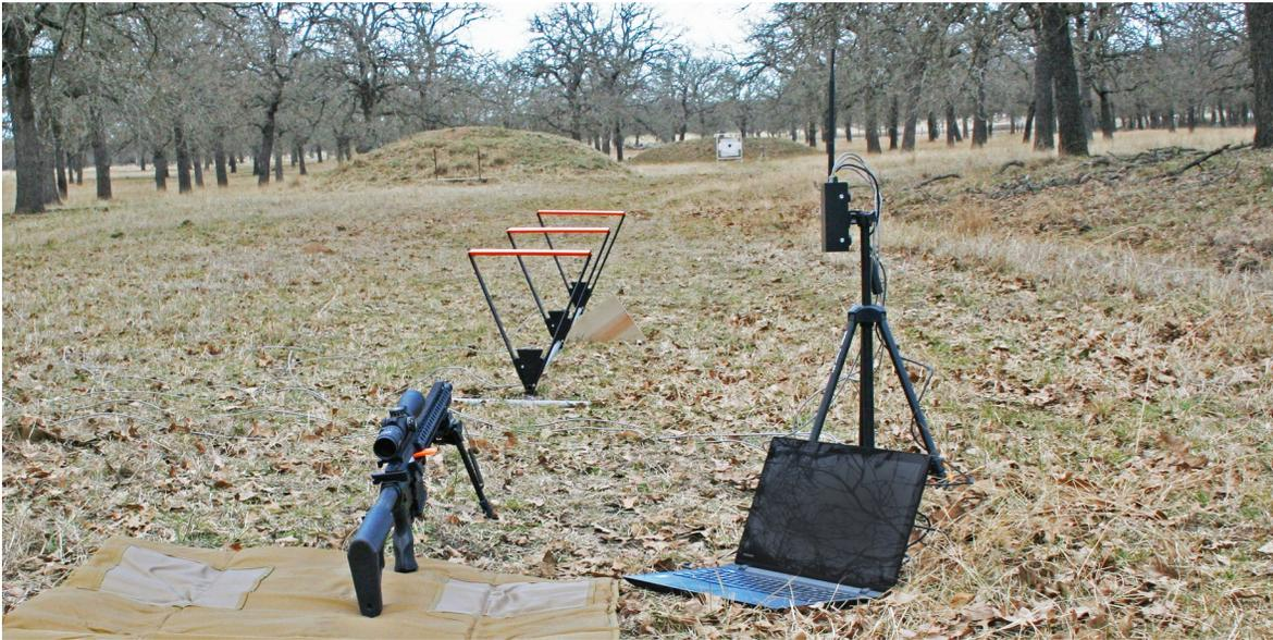
A conventional chronograph only measures velocity near the muzzle. The BC Chrono™ System measures both muzzle velocity and the time-of-flight from gun to distant target. An accurate ballistic coefficient requires both measurements. The System 89 makes both measurements and computes the exact BC for your ammo and your gun.
