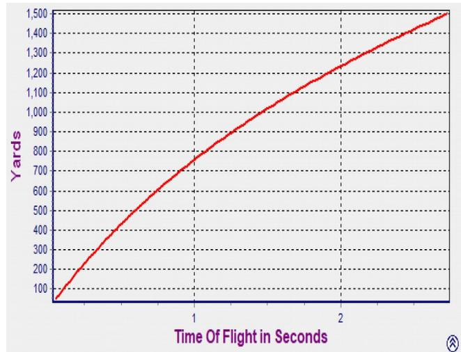
For example, here is a red curve illustrating the distance traveled versus time for a bullet having a G1 ballistic coefficient of 0.500 and launched at 3000 feet per second. It's simple, but tells much.
