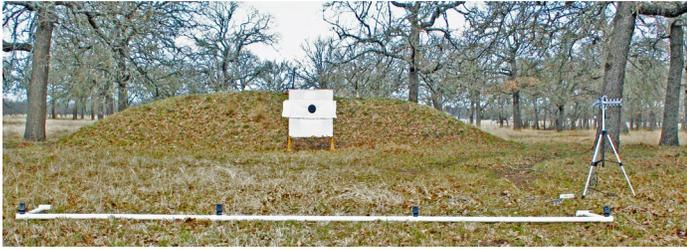
The easiest target array to use has the four microphones lined up on the ground perpendicular to the bullet's expected path. An array 15 feet long will typically detect bullets passing within 10 feet of the array.
