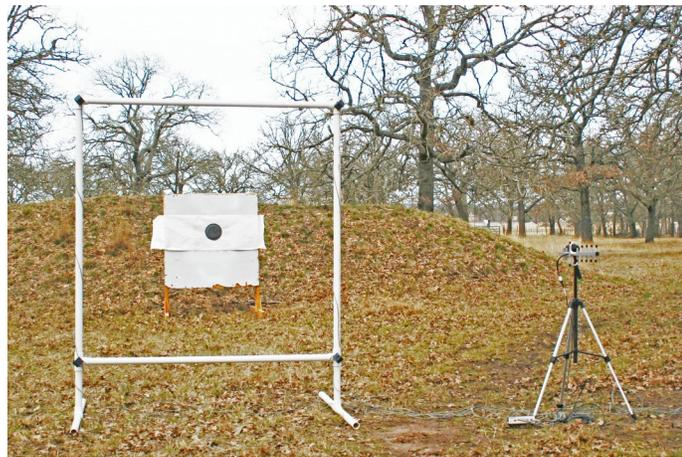
A square *fly-thru* array may be used for increased scoring accuracy. You get better scoring, but it is more difficult to set up and you have a smaller window. The maximum size of the square is 10 feet.
