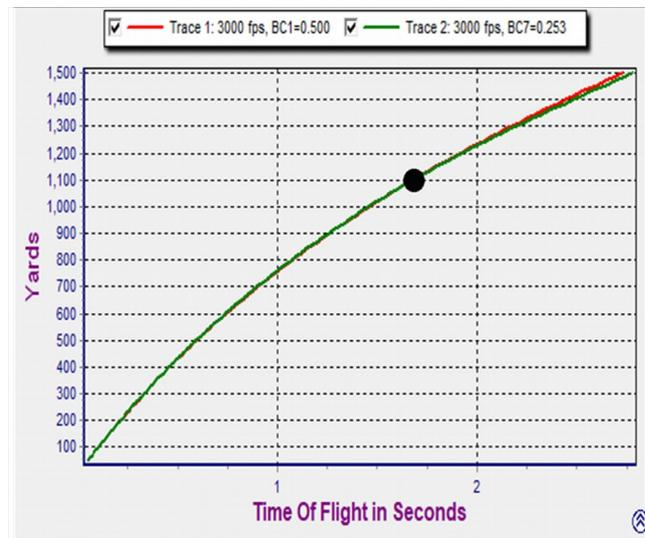
Here are two distance versus time curves using G1 and G7 at the same muzzle velocity. We choose the ballistic coefficients so that times-of-flight match at 1100 yards. The green G7 curve completely obscures the red G1 curve out to approximately 2 seconds or 1200 yards. The difference in zero-adjust remains less than 0.1 mil out to 1350 yards where the bullet has fallen subsonic.
