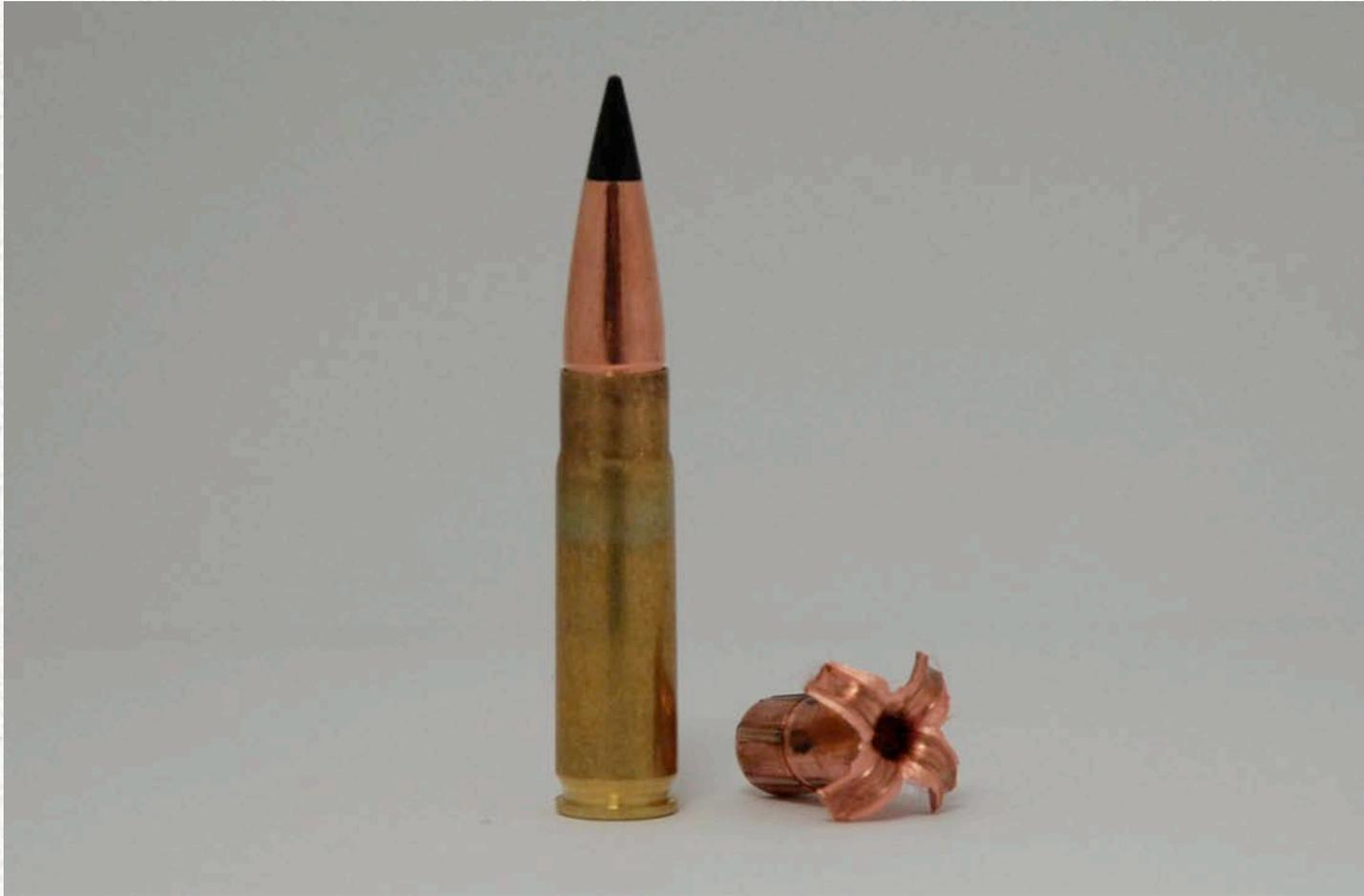
20 inches of penetration at 300 yards (275 meters) from 9 inch barrel
